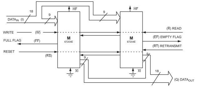
**Note :** 3. Flag detection is accomplished by monitoring the FF, EF and the HF signals on either (any) device used in the width expansion configuration. Do not connect any output control signals together.
