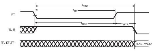
**Notes :** 23.  $\overline{EF}$ ,  $\overline{FF}$  and  $\overline{HF}$  may change status during Retransmit, but flags will be valid at  $t_{RTC}$ .
